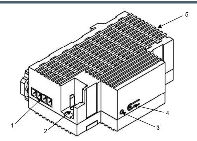
Programming button: a push button to set programming mode. If this button is held while plugging the device into the KNX bus, it goes into secure mode.
